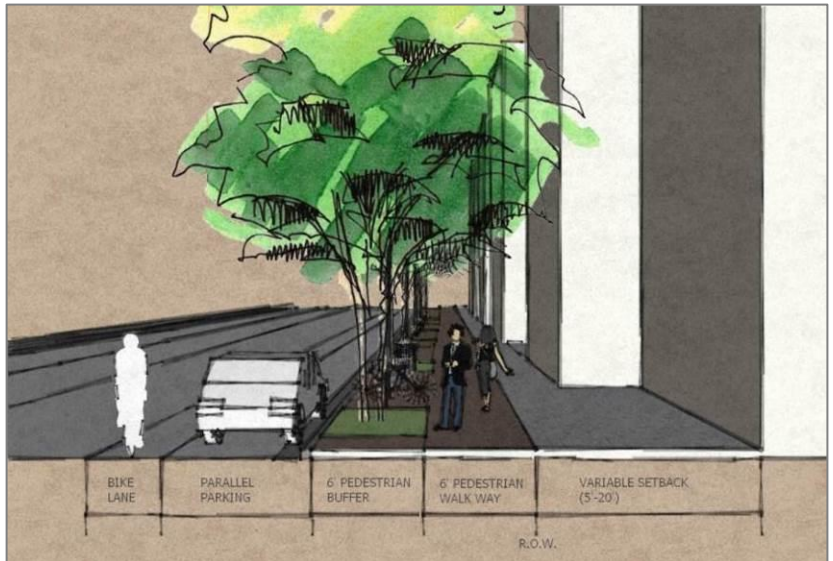
Figure 29: Main Street Sidewalk (Typical Section)
